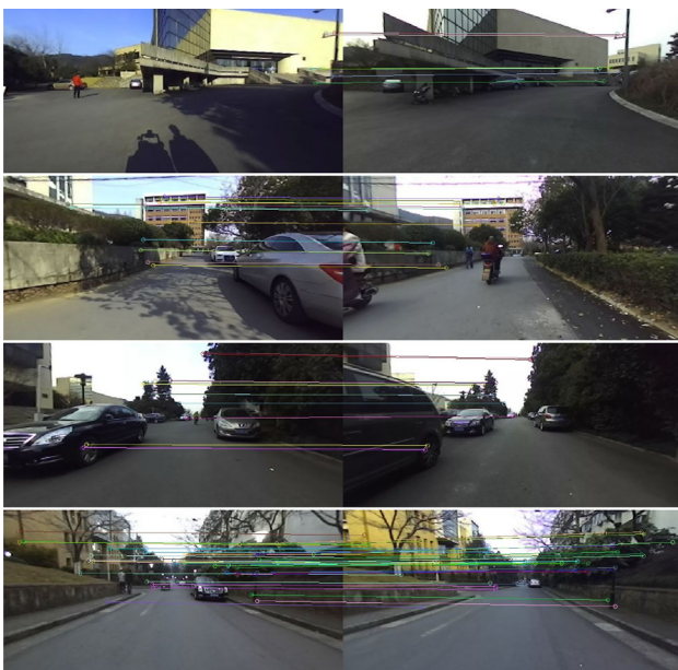
Fig. 12 Cases of feature points matching. Row 1 to 3 present 3 examples of failure case, while row 4 is a successful one
