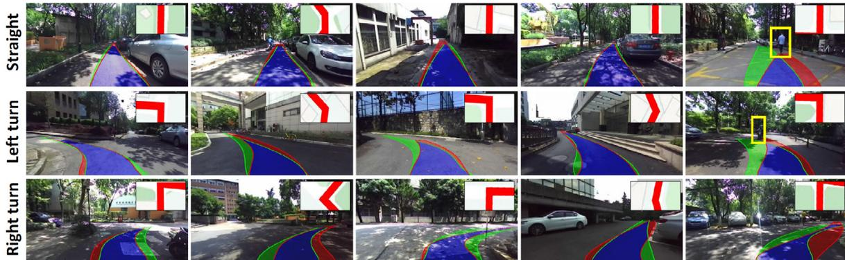
Fig. 10. Visual results from cGAN-LSTM. Green, red, and blue colors represent prediction, human demonstration and their intersection respectively. The local route plans are shown in the top right corner of the image. The intention boundaries are fitted with splines in these figures. (For interpretation of the references to color in this figure legend, the reader is referred to the web version of this article.)
